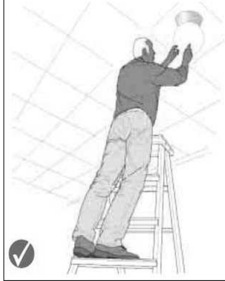
Correct – 3 clear rungs, do not work any higher on this type of stepladder
