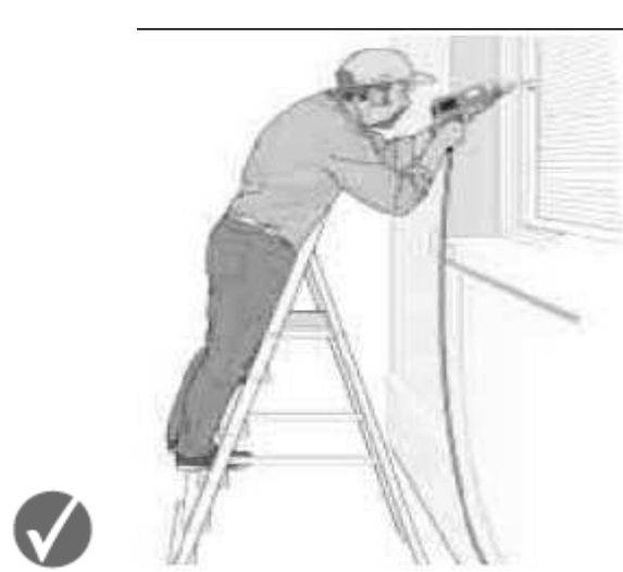
Correct – steps facing work activity
