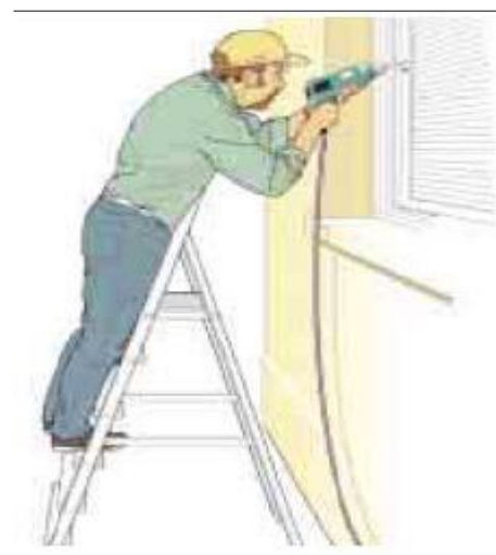
Correct – steps facing work activity
