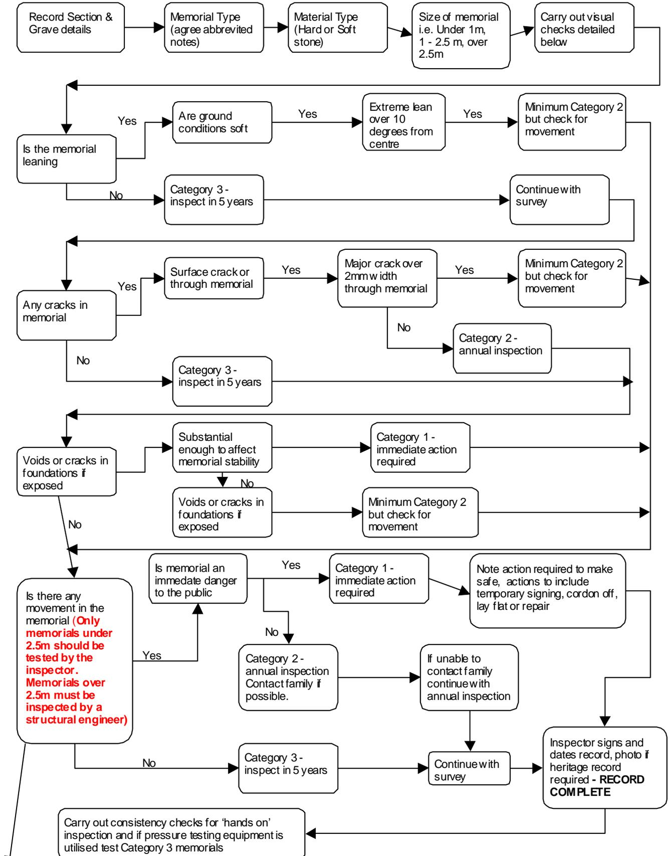
**NOTE:** Full visual inspection only is made of memorials over 2.5 metres in height. Where visual inspection indicates that a problem may exist the inspector should take immediate action to cordon off pending full inspection by structural engineer. Structural engineer must inspect all memorials over 2.5 metres in height commencing with those identified by the inspector as possibly posing a hazard.
