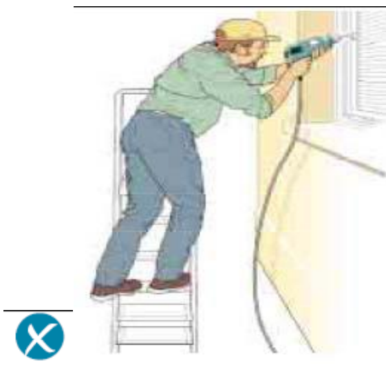
Incorrect – steps side on to work activity
