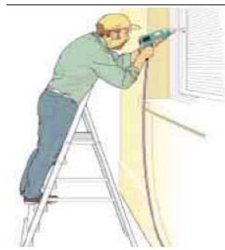
Correct – steps facing work activity
